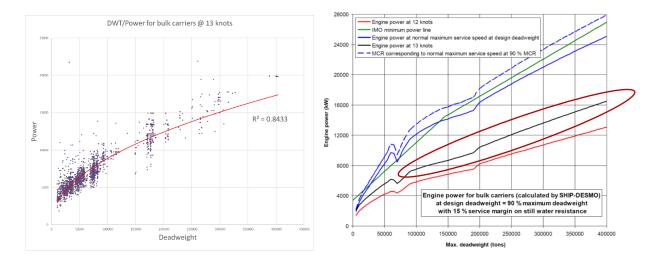
14 Comparing the Deadweight/Power at 13 knots regression curve, using IHS Fairplay data, with the result of the Danish Technical University's SHIP-DESMO generic computer model for bulk carriers' power at 13 knots versus deadweight shows a reasonable fit. This suggests that using the IHS Fairplay database to derive the required power limit curve may be feasible, subject to further examination for any applicable ship type.
